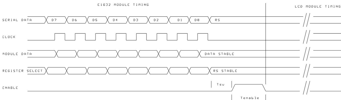
**Figure 2. E1832 Signal Timing**
