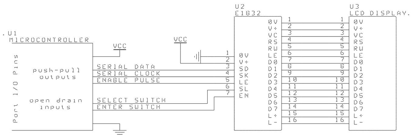
**Figure 1. E1832 Module Connection**
