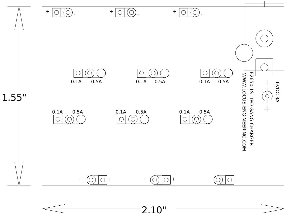
Figure 1. Module Dimensions
