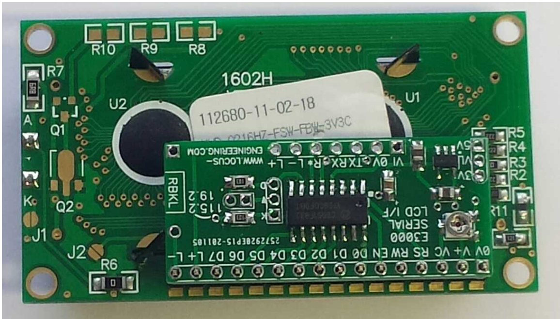
Figure 4. E3000 module on bottom mounted 1x16 LCD connector.
